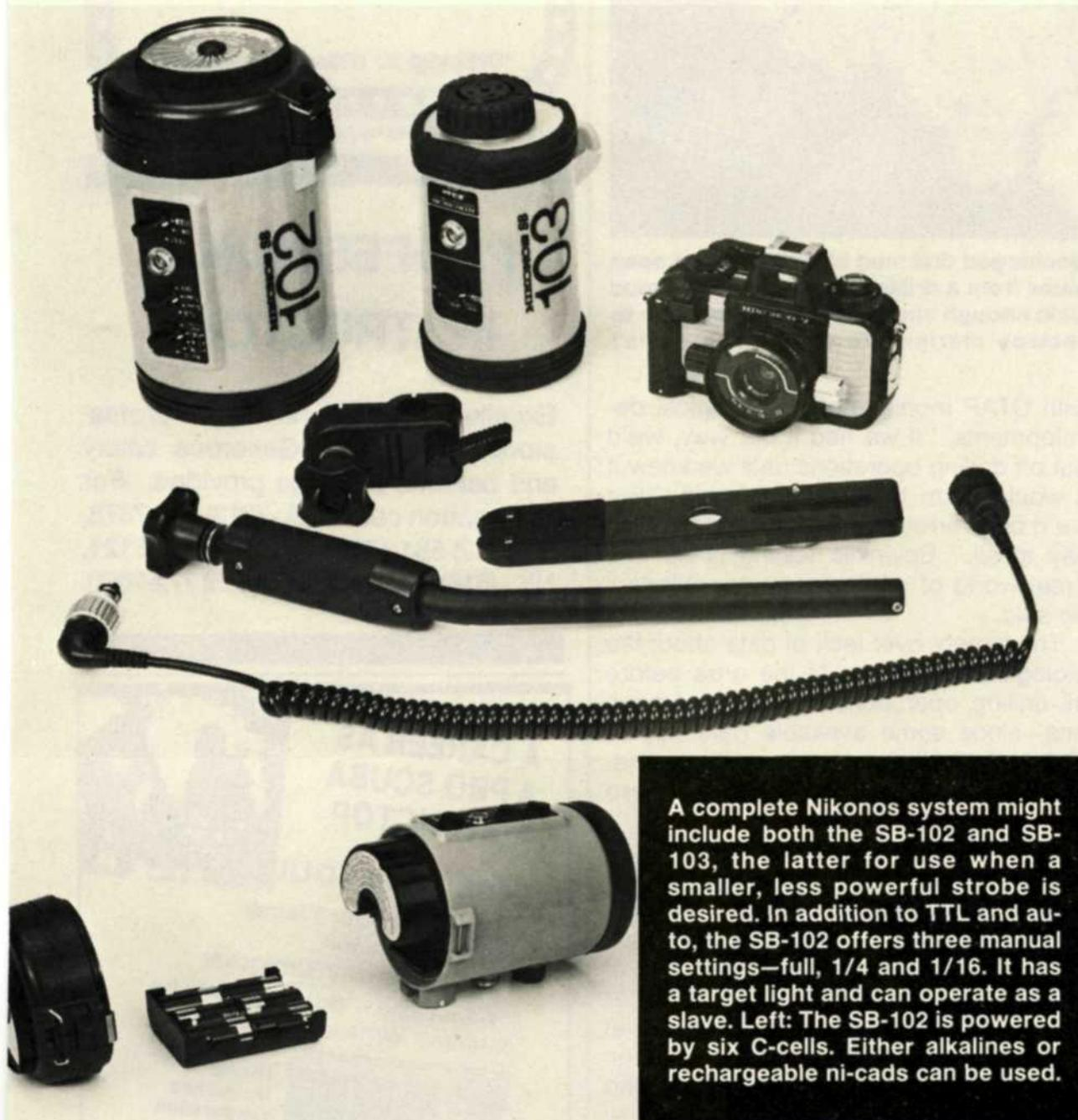
A complete Nikonos system might include both the SB-102 and SB-103, the latter for use when a smaller, less powerful strobe is desired. In addition to TTL and auto, the SB-102 offers three manual settings—full, 1/4 and 1/16. It has a target light and can operate as a slave. Left: The SB-102 is powered by six C-cells. Either alkalines or rechargeable ni-cads can be used.
